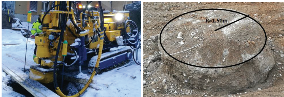
Figure 8 & 9. ACI testing (on the left), physical result of the Keller ACI test (on the right)
