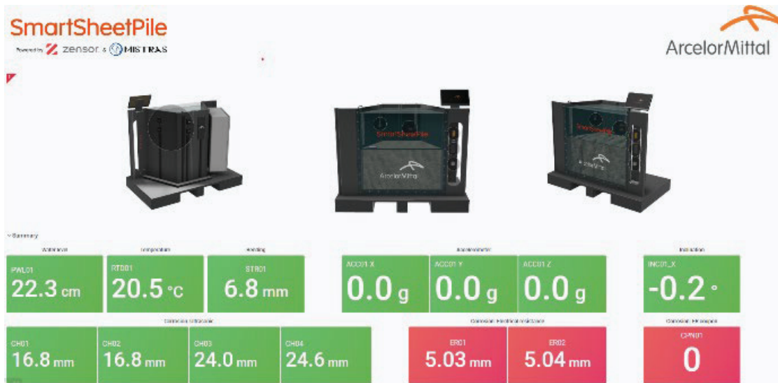
Figure 5 The main interface of the online dashboard of the demonstrator including its digital twin model.
