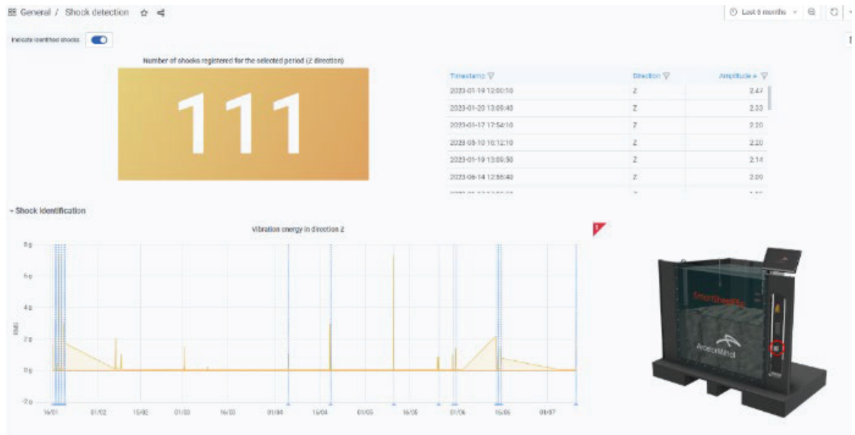
Figure 6 Example of the online dashboard features: Overview on the Shock detection sensor of the demonstrator during the last six months.
