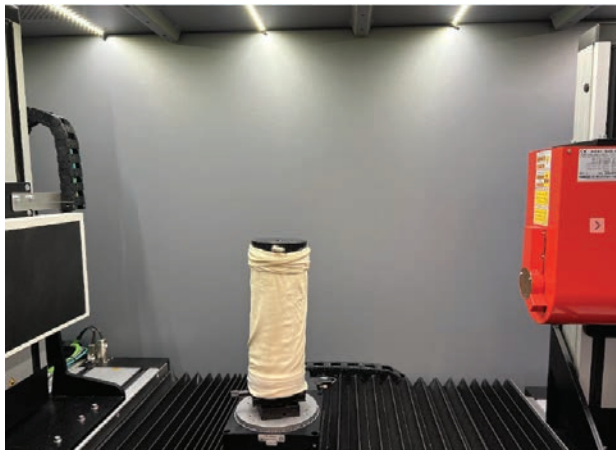
Figure 2 Image acquisition via x-ray tomography
